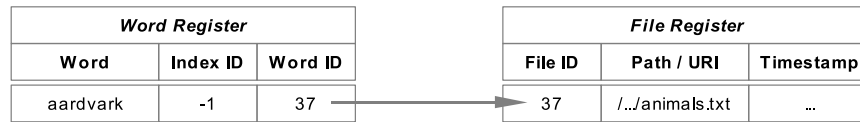
Figure 4: In this example, the word 'aardvark' is directly linked to the only file it appears in. For this case no intermediate lookup tables are needed.
